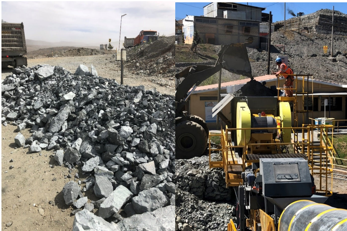
Figure 3 - Line dumping of ore next to the bulk ore sorting plan and loading of feed to the crusher.
